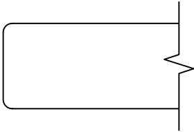
Eased Edge (R3) Internal Lumber Band
