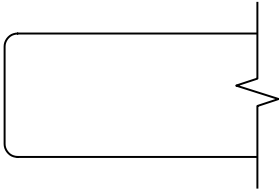
Eased Edge (R3) Internal Lumber Band
